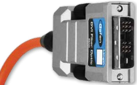
Fiber Optic based cables that exceed the performances of the copper and silver made cables. An integrated DVI-D cable solution which includes the fiber optics components built into the cable and the DVI connectors. DVI Fiber Optic cable requires a clearance of 1-1/2" wide conduit. Available in lengths of 33-330 feet. These cables are for computer use only.
