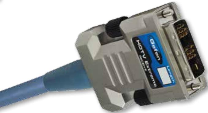
An integrated DVI-D cable solution which includes fiber optic components and DDC circuitry built into the cable assembly. Requires a minimum 1 1/2" conduit for clearance. These cables are HDCP compliant.
